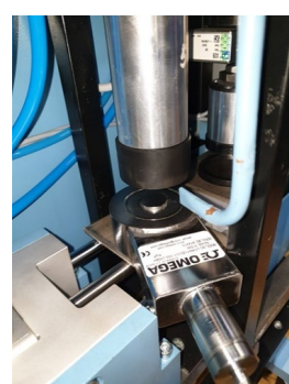
Calibration load-cell placed on top of adapter plate.
