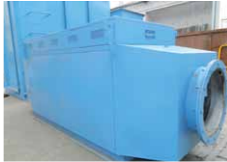
Gas fired heating systems for ducts
