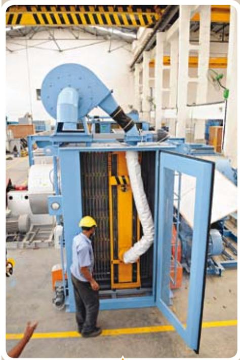
Dust filters: Reverse air cleaning using RA Fan instead of compressed air
