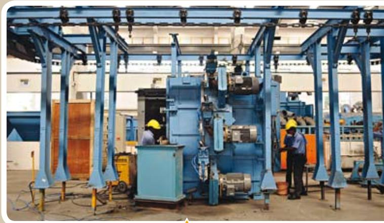
Shaping the future of foundry: Fully automatic Shot blast machine (SBM) will make surface cleaning much easier and faster.
