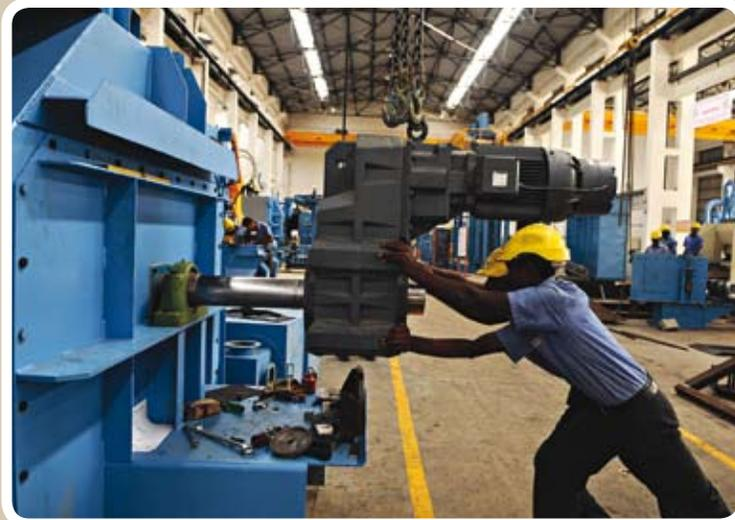
De-assembling machine in order to ensure easier and safer transportation
